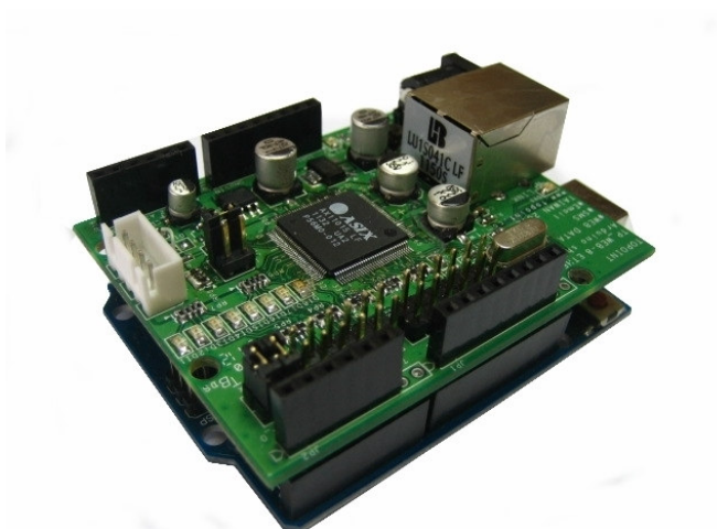
TP-ESMS-8 Board is stacked on Top of Arduino Uno Rev2
